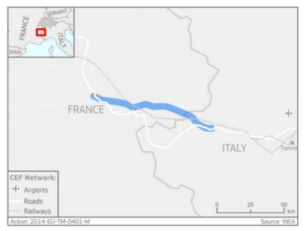
The existing railway line from France and Italy runs through the Alps with heavy rail traffic. However, it is a mountain line which has limited traffic performance. The Action will develop a new rail network between France and Italy for wide gauge (heavy freight), rolling motorway and high speed passenger trains. It is part of a Global Project on the development of a crossborder rail network to link Europe from east to west. The Action forms a key part of the Mediterranean Core Network Corridor.
